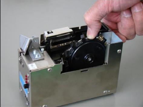
A photograph showing a person's hand holding a finger against a black rotating drum of a metallic device. The device has a silver-colored metal casing and a blue component on the left side. The hand is positioned to lock the drum in place for adjustment. |
